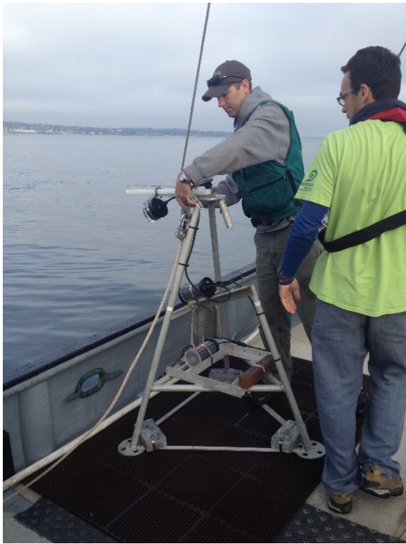
Deploying the “Sea Star” video system, developed by the Monterey Bay Aquarium Research Institute, to monitor squid egg beds.
